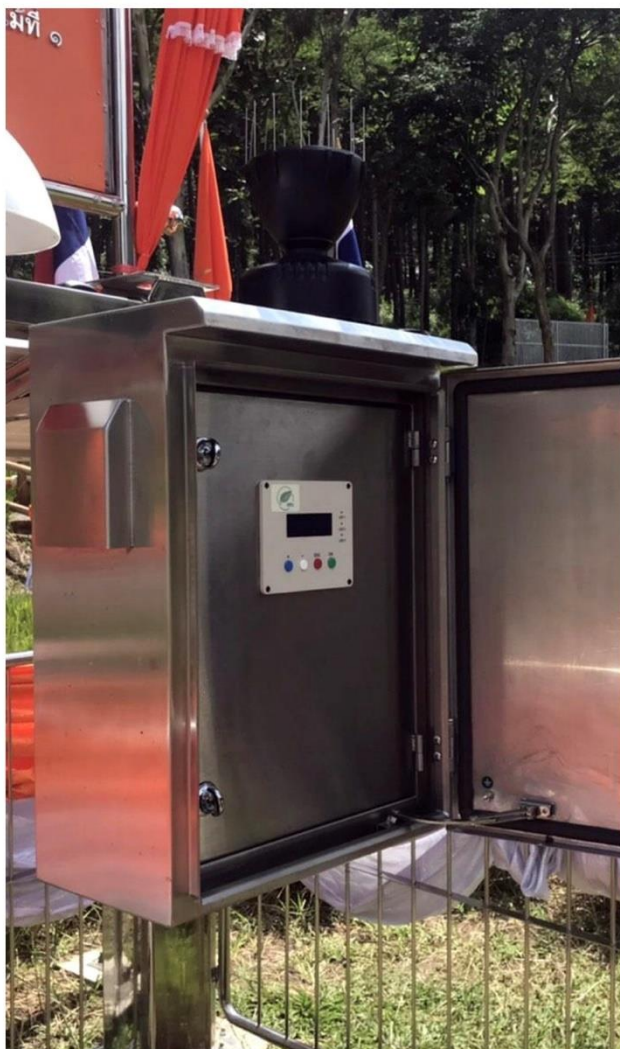
Photo: (from left to right) Automated Telemetry Station in Pongyeang sub-district, Mae Rim District, Chiang Mai Province and interface of ThaiWater mobile-application that has been integrated for general use.
